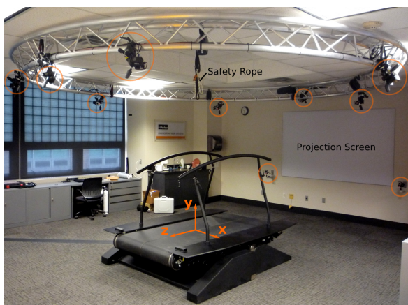
FIGURE 5.1: The setup of the experiment. The vertical direction is defined as y , anterior/posterior direction as z and the mediolateral one as x . Figure adopted with permission from Moore 2015 (CC-BY-4.0) [129].
